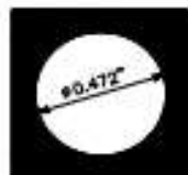
PANEL DRILLING Ø0.472"
