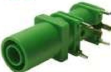
FCR7370G - S16N-2PC Green 4mm shrouded socket. Gold plated Rated: 1KV CAT III - 10A
